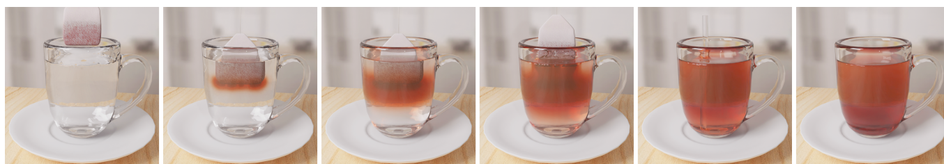
Fig. 1. Tea diffuses from a teabag into a cup of water. After the teabag is removed, the mixture is stirred with a (glass) rod.
