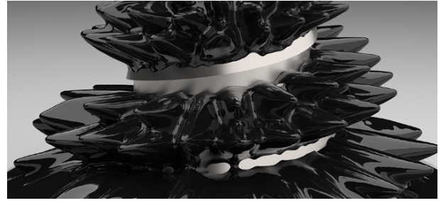
Fig. 48 A ferrofluid climbs up a steel helix under a strong external upward magnetic field to create surface spikes [305].
