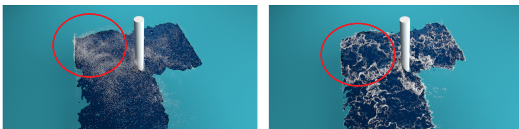
Figure 11. Comparisons of the experimental results without considering coupling parameters ( left ) and our method ( right ). The 80th frame of a dam burst collides a static cylinder. Considering the coupling parameters, the diffuse material is more in line with the fluid boundary, the experimental effect is more realistic.
