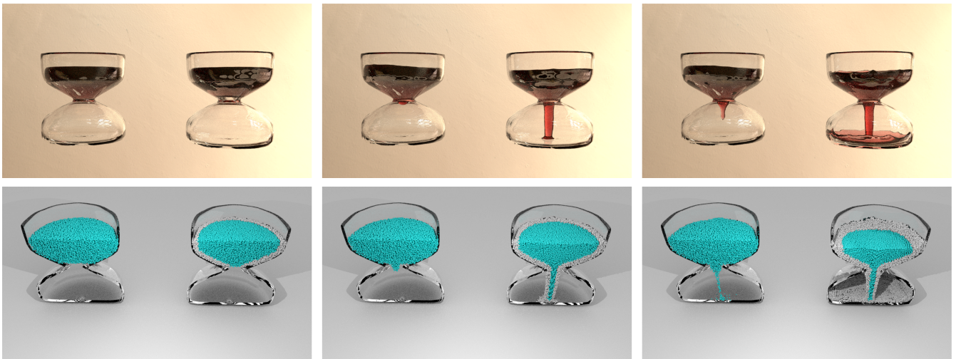
FIGURE 6 | Fluid flow in an hourglass. We use blue color for original particles and white color for subdivided ones. Comparing with the results of the original grid (left), our adaptive method (right) allows the fluid to pass through fine apertures smoother.
